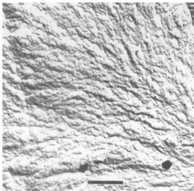
Figure 8 Transmission electron micrograph of a replica of fracture surface of copolyamide annealed at 240°C and 6.5 kbar for 40 h. Scale bar represents 1 \mu\text{m}
